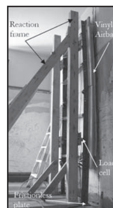
(b) Typical test setup for one-way bending (Avon House)
