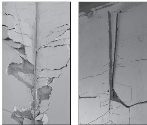
(a) Debonding (b) Sudden pull-out
