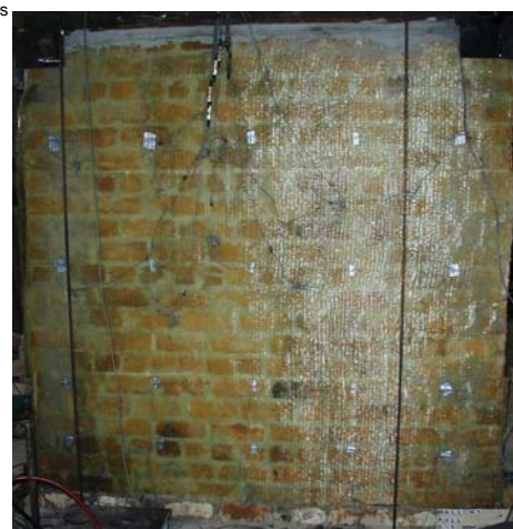
(b) FRP-retrofitted wall
