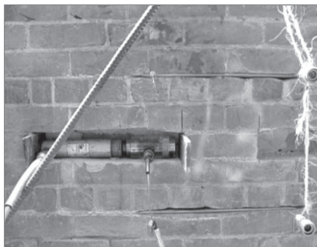
Figure 4. Typical mortar bed joint shear test setup
