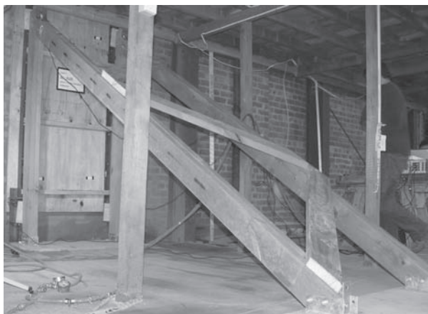
Figure 15. Reaction frame for out-of-plane test
