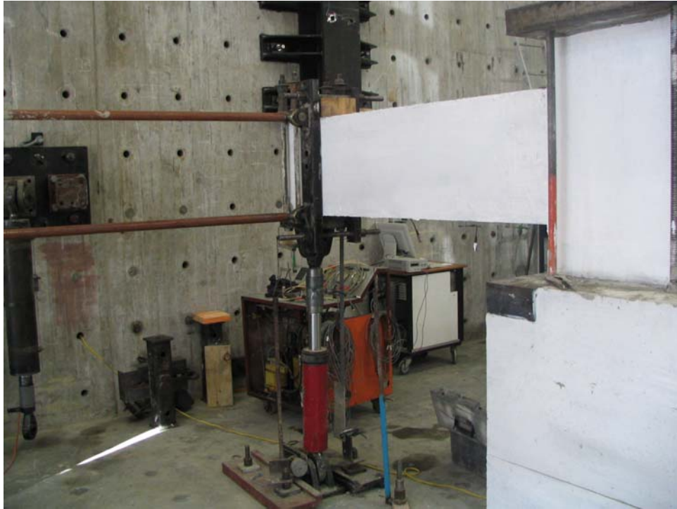
Figure 4 Torsional Restraint System and Jack Setup for Unit 1
